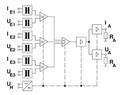
notice: Input, outputs and auxiliary voltage are galvanically isolated from each other.
